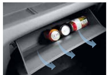
Glove box cooling
